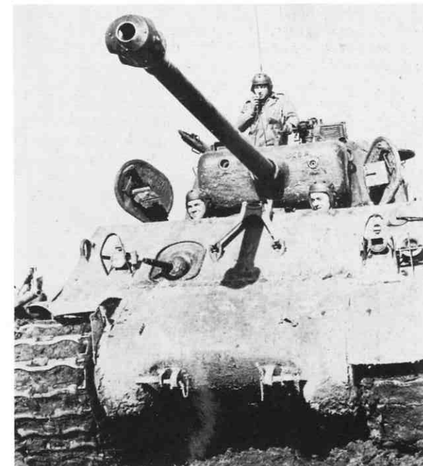
▲ The Americans had some upgraded Shermans called 'Cobra Kings' armed with 76mm guns with muzzle brakes and having thicker frontal armour. Patton ordered that they lead the effort to break through to Bastogne. (US Army Military History Institute)
